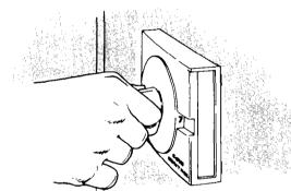
Before loading with unfrozen food, turn cold control to coldest position (highest number) and let freezer operate for several hours. This will speed up the rate of freezing. Lay packages to be frozen in a single layer so each rests on the freezing surface of a shelf. Allow space between packages for cold air to circulate.
